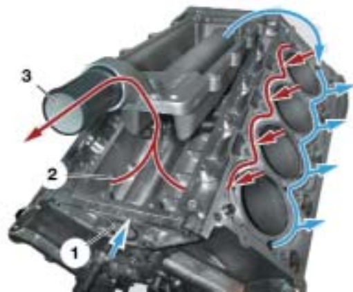
Engine Block Coolant Flow
